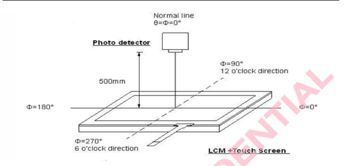
Fig. Optical measurement system setup
